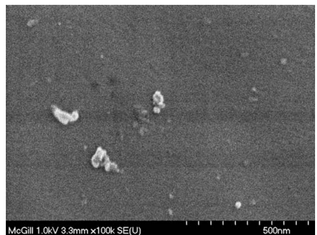
Fig. 3 Surface of the conventional YSZ powder
